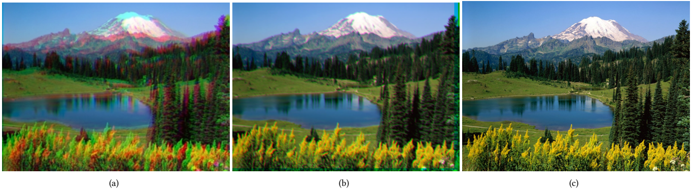
Fig. 5. (a) A synthetically aberrated mountain image via translation in different colour channels. (b) A corrected version using our algorithm. (c) The ground truth image.
