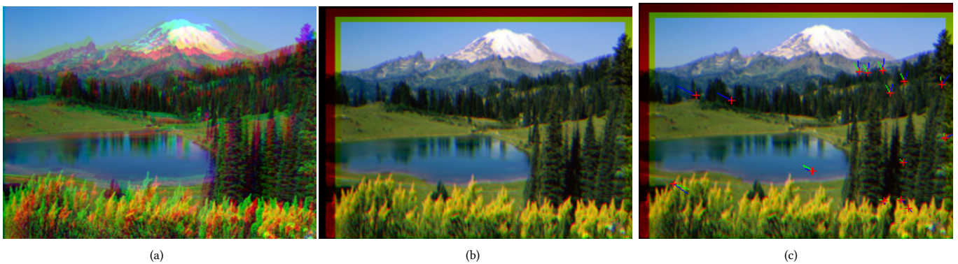
Fig. 6. (a) An image with exaggerated translation and scale shift in two colour channels. (b) A corrected version using our algorithm. (c) The same corrected version showing disparities and keypoints.
